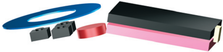
Figure 17 - Quick render to portray parts in their position. Touch wheel, three buttons below, vibrating motor in red, battery in pink, logic board in black, with standard 3,5 mm audiojack.
